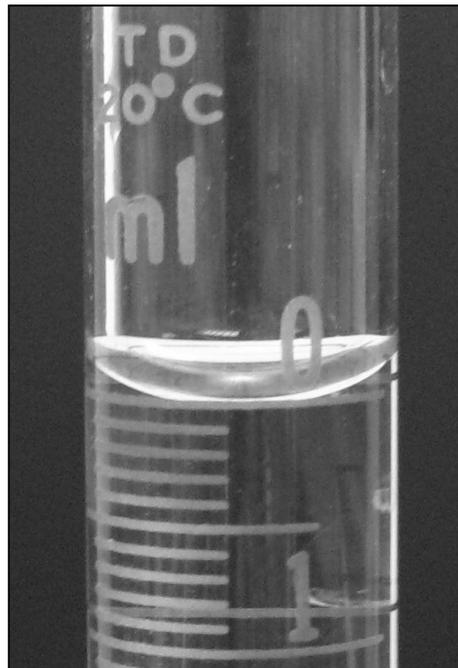
**Reading the Burette:** Burette reading involves reading all of the marked lines [ ml and tenths of an ml ] and interpreting the reading between two lines for the 0.01 ml reading.
